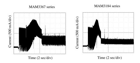
Figure 4.8 Current waveform (+12 VDC)
